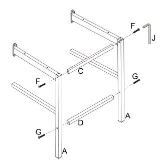
Attach the Chair Frame L & R (A) to the Chair Back (B) using Bolt (G & H) with the Allen Key (J).
