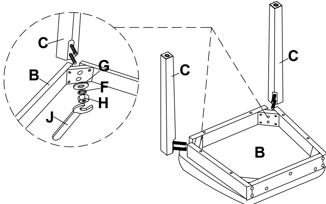
Take the Allen Wrench and turn the bolts until the legs are secured.
