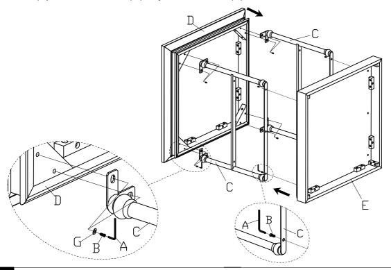
2 Assembly the Shelf(F) onto the Side Frame(C) and using the Bolt(B) by Allen Wrench(A).
