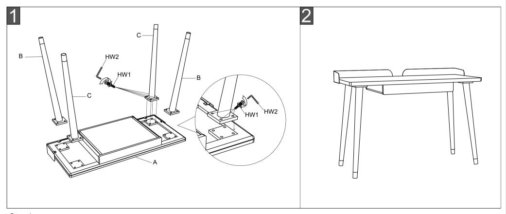
Step 1: Assembly 2\*Leg-1 (B) to the underneath of the table top (A) in diagonal position facing front left. Using Allen key (H2) to lock with 8\*Hex Socket Bolts (HW1). Repeat this process to assembly rest 2\*Leg-2 (C). As picture.
