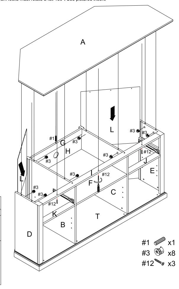
Step 8. Secure back panels (part L) to top panel (part A) using round head screws (part #10) and phillips head screwdriver.
