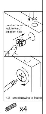
Step 3. Attach right vertical panel (part C) to assembled unit (parts F, G & H) using wood dowels (part #1) and cam locks (part #3).
