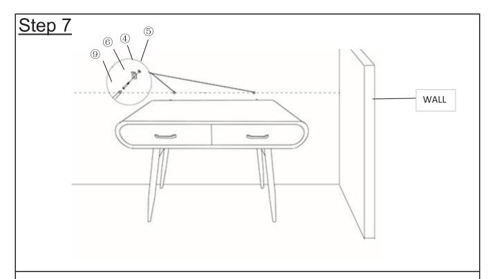
Attach Metal Bracket(4) to Wall Plug(5) using Wall Plug Screw(6) with Screwdriver(9).
