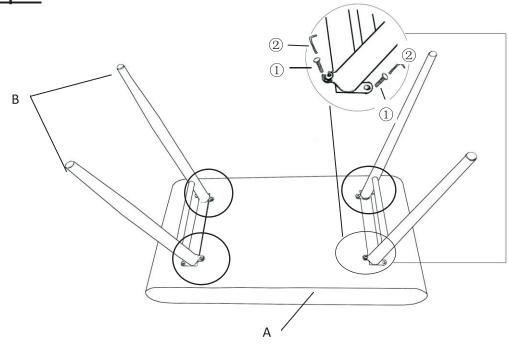
Insert the Leg into the leg position in the Table Top(A). Attach the Leg(B) to the Table Top(A) using Bolt(1), with Alley Key(2).
