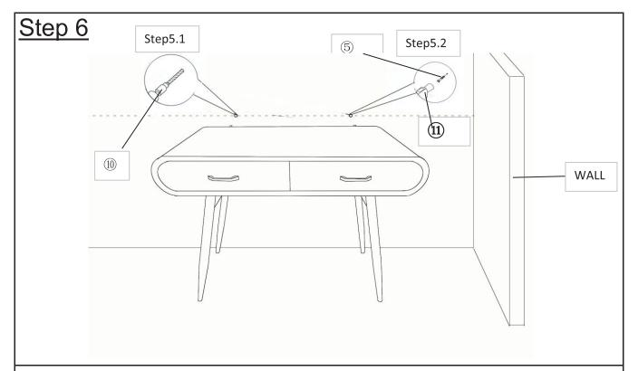
6.1) Drill two mounting positions on wall at same height as Metal Bracket(4) on Table back with Power Drill(10).
