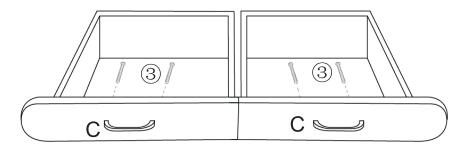
Attach the Handle(C) to the drawer of Table Top(A) using Bolt(③) with Screwdriver(⑨).
