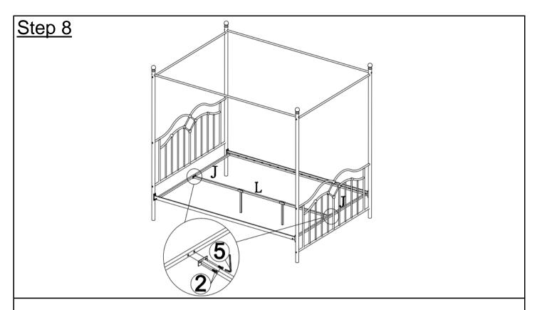
Turn over the assembled Center Support Rail(L&M). Attach assembled Center Support Rail(L&M) to Support Rail(J) using Bolts(②) with Allen Key(⑤).
