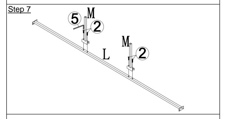
Attach Support Leg(M) to Center Support Rail(L) using Bolts(2) with Allen Key(5).
