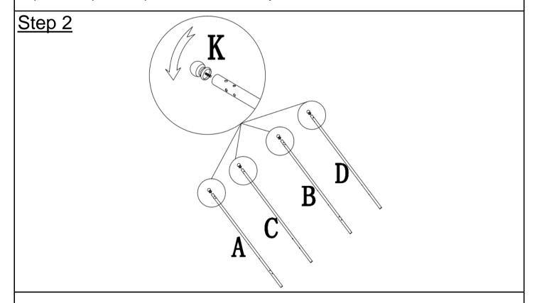
Attach Finials(K) to mounting positions on Left Headboard Post(A), Right Headboard Post(B), Left Footboard Post(C) and Right Footboard Post(D) by turn clockwise by hand.
