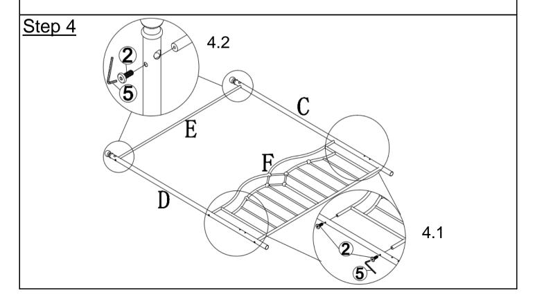
**4.1)** Attach Left Footboard Post(C) to Headboard/Footboard(F) using Bolt(2) with Allen Key(5).
