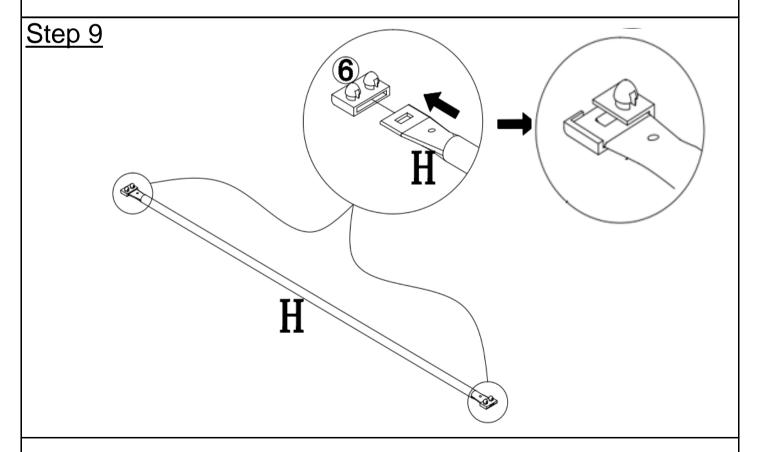
Insert Slat Connectors(6) into both sides of Slat(H) as pictured above.
