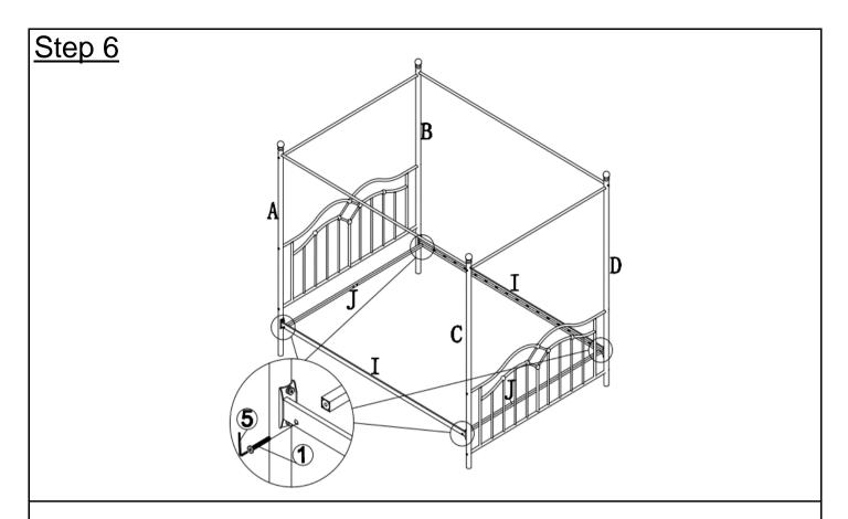
Attach Support Rail(J) to Side Rail(I) using Blots(1) with Allen Key(5).
