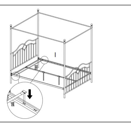
Attach assembled Slat(H) to the mounting position of Side Rail(I).
