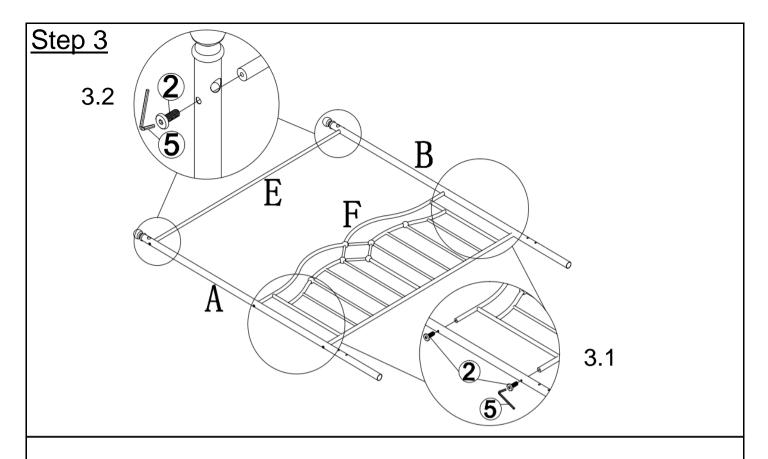
**3.1)** Attach Left Headboard Post(A) to Headboard/Footboard(F) using Bolt(②) with Allen Key(⑤).
