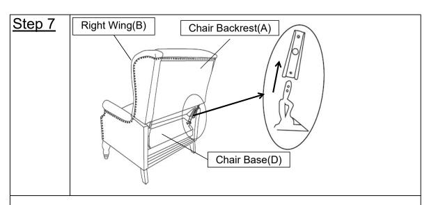
With assistance from your adult partner, hold up the fully assembled Chair Backrest(A) with Right Wings(B) and Left Wing(C), stand behind the chair. Insert the small metal arms on the sides of the Chair Backrest(A) into the prefabricated slide lock gadget on the Chair Base(D) as shown above. Firmly but gently, push the Chair Backrest(A) downwards until the Chair Backrest(A) is fully slotted and locked into position.
