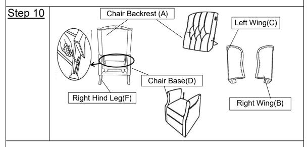
Disassembly Note:Open the flap on the Chair Backrest(A),use a screwdriver(Don't use fingers) pressing outward on the metal ear on the preattached Metal Bracket on one side of the Chair Base(D),with assistance of you adult partner to keep the Chair Base(D) in place, pull out the Chair Backrest(A) upward at the same time,repeat the same step for another side. Then the Chair Backrest(A) can be taken out.
