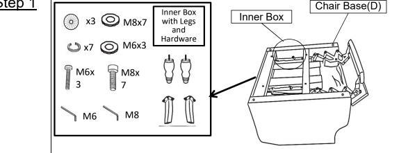
Place the Chair Base(D) facedown on a clean, non-marring surface. Take out the four wooden legs and Hardware from inner box, as picture shown on above.
