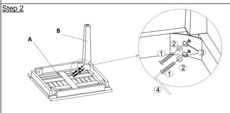
Attach Leg (B) to Table Top (A) by using Bolts(1), Flat Washer (2), Spring Washer (3) with Allen Key (4).
