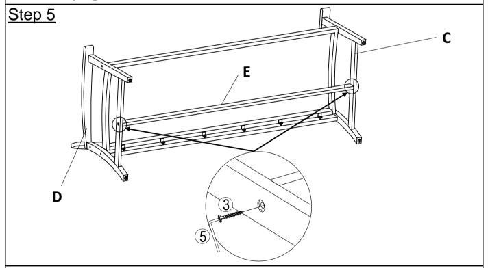
Insert Leg Support Bar (to Right Leg Panel (C) and Left Leg Panel (D) using Screw (3) with Allen key (5) as shown above.
