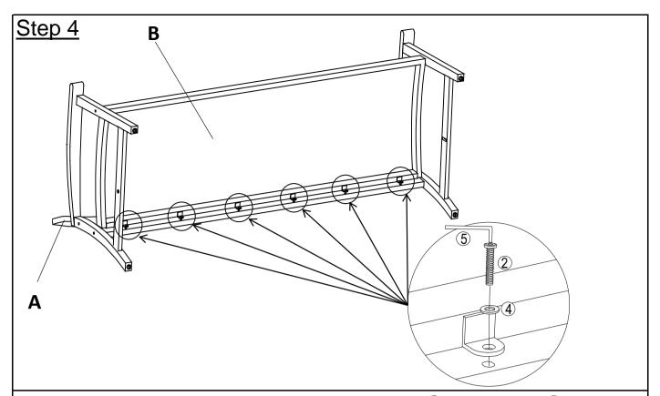
Secure Seat Panel (B) to Back Panel (A) using Bolt (2) & Washer (4) with Allen key (5)
