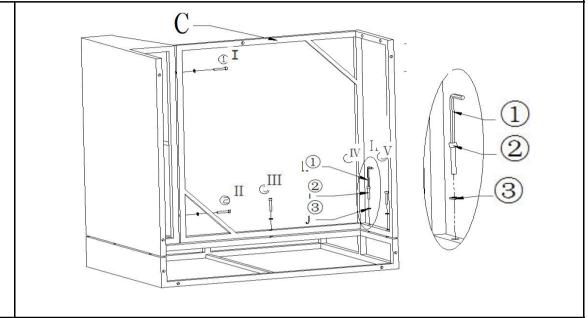
Attach Seat(C) between the Right Armrest(A) and Back(B) using Bolt(②) and Washer(③) with Allen Key(①) from position # I to # V as shown above.
