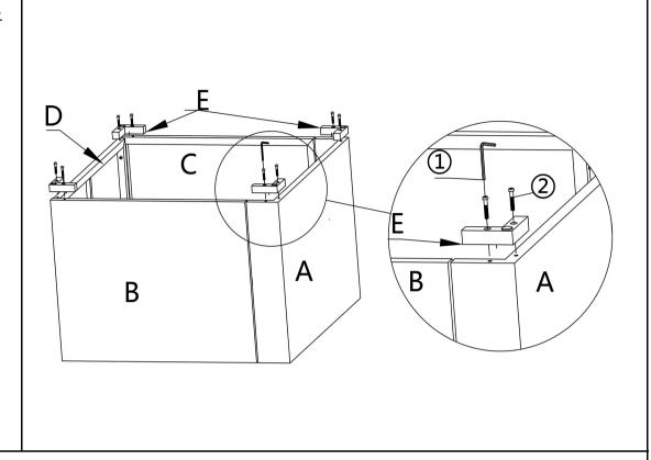
Attach the Foot(E) to the Chair using Bolts((2)) with Allen Key((1)).
