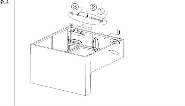
Attach Side Plate(D) between the Back(B) and Seat(C) using Bolt(2) and Washer(3) with Allen Key(1) as shown above.
