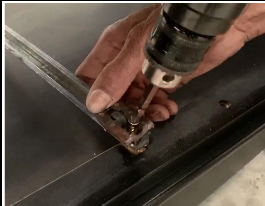
Step 9 Lock it in with a wooden screw, fix it.
