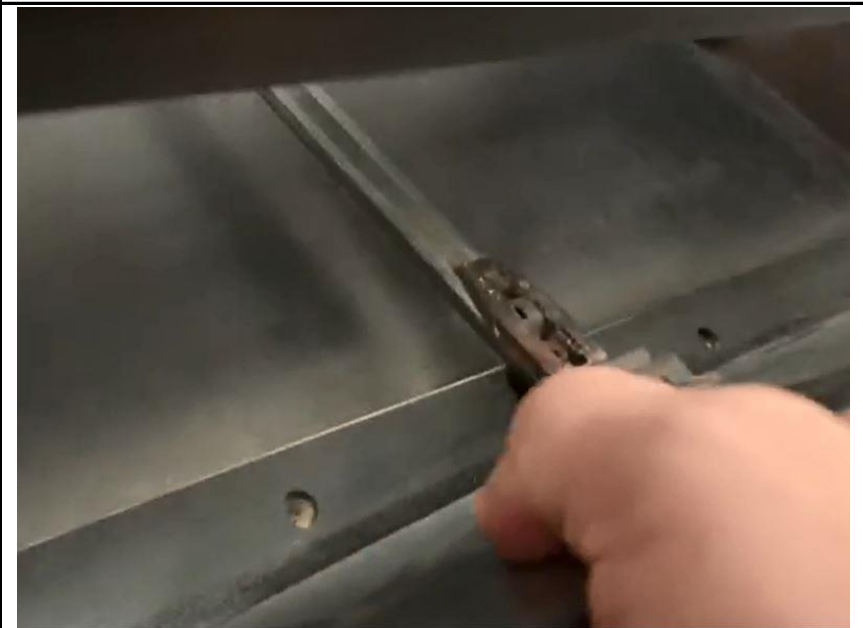
Step 11 fit the male metal glide and female groove (Make sure the male glide is aligned with the female groove)
