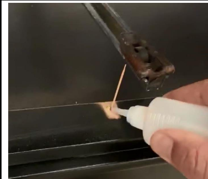
Step 7 Repeat the previous method/step, to insert the toothpick into the hole and run into quick-drying adhesive
