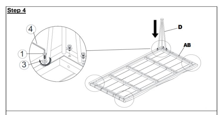
Attach Leg (D) to Side Table Top (B) using Bolt (1) and Washer (3) with Allen Key (4) as shown in above picture.
