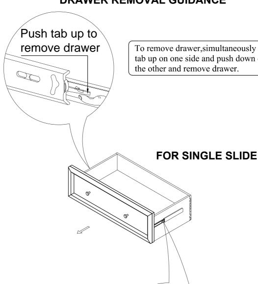
To remove drawer, simultaneously pull tab up on one side and push down on the other and remove drawer.
