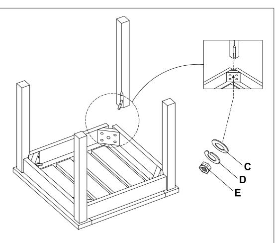
Attach the leg (B) into each corner of table top (A). Insert washer (C), spring washer (D), and nut (D) to each leg (B). **Tighten nuts using wrench.**
