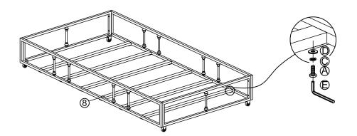
NOTE: DO NOT TIGHTEN ALL THE BOLTS UNTIL THEY ARE INSTALLED IN CORRESPONDING HOLES!
