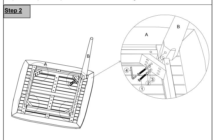
Attach Leg (B) to the Table Top (A) by using 2 Bolts (1), 2 Spring Washers (2) and 2 Washers (3) with Allen Key (4).
