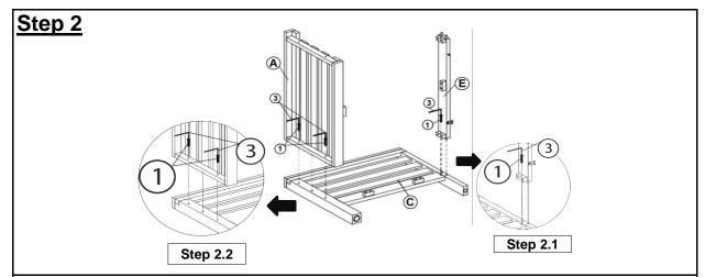
Place the Right Arm Panel (C) with inside face skywards onto a clean, soft surface to avoid any scratches or damages to the product. Step 2.1: Align the dowels of Support Bar (E) into the positions in the Right Arm Panel (C).
