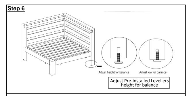
Inspect the Chair and make sure all parts are adequately connected. In a sequential manner, tighten all Screws and Bolts at all joints. With assistance from your adult partners, adjust the Levellers to desired height to avoid wobbles.
