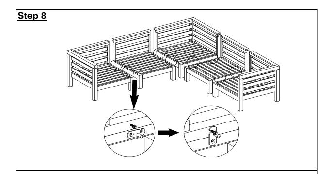
Note: This is optional step in case we want to connect all chairs in a set together and should be done before placing cushion With assistance from your adult partners, up side down the chairs and using pre-fixed clip to connect the chairs together
