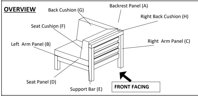
This Right Chair has multiple parts and may require up to 30 minutes to assemble. To give you an overview of the Right Chair parts, the above picture is to help you put the various parts into perspective. Please read through the instructions herebelow to familiarise the parts and steps before assembly.
