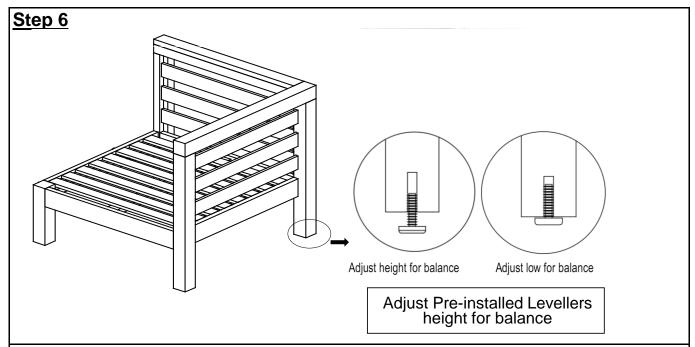
Inspect the Right Chair and make sure all parts are adequately connected. In a sequential manner, tighten all Screws and Bolts at all joints.
