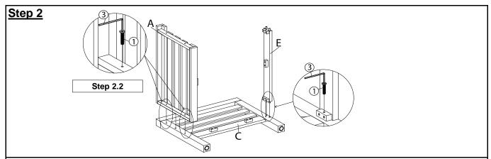
Place the Right Arm Panel (C) with inside face skywards onto a clean, soft surface to avoid any scratches or damages to the product.
