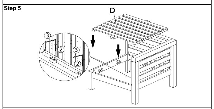
Attach the Seat Panel (D) into the Right Chair as shown in picture above. Affix Seat Panel (D) with Corner Chair by using Screws (2) and Allen Key (3). Note: Using Screws (2) from inside to outside of Seat Panel (D)
