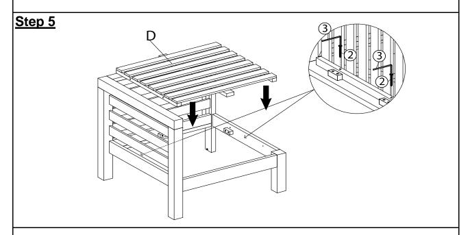
Attach the Seat Panel (D) into the Chair as shown in picture above. Affix Seat Panel (D) with Chair by using Screws (2) and Allen Key (3). Note: Using Screws (2) from inside to outside of Seat Panel (D) **DO NOT FULLY TIGHTHEN SCREWS.**
