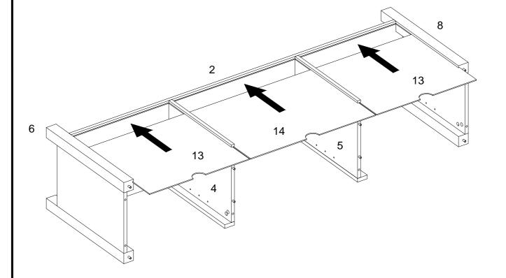
Slide the back panel all the way into the groove
