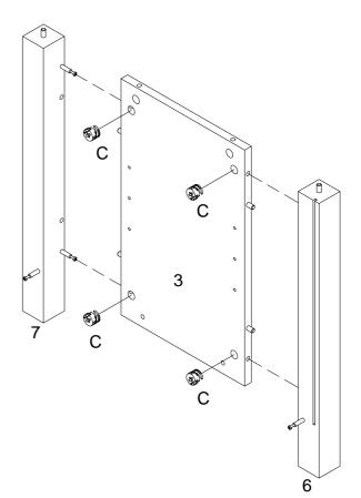
Attach part 3 to part 6,8,9 with cam lock (C)
