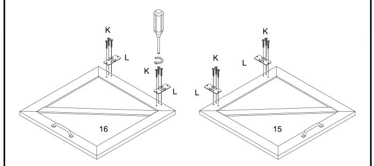
Attach door hinge (L) to part (15,16) using screw (K) with screwdriver.
