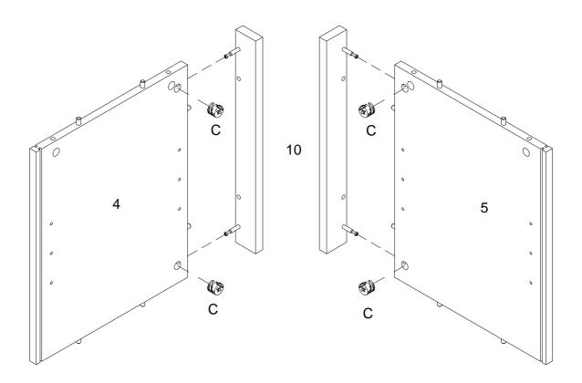
Attach parts (4,5) with cam locks (C)
