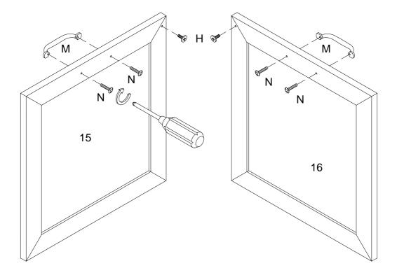
Attach handle (M) to part (15,16) using handle bolt (N) with screwdriver.
