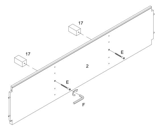
Attach part (17) to part (2) using bolt (E) with hex key (F).
