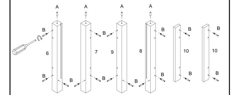
Secure cam bolt (B) with screwdriver into part (6,7,8,9,10), insert wooden dowel (A) into part (6,7,8,9)
