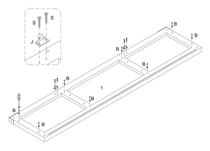
Secure the Door Stopper (J) with Screw (S) and cam bolt (B) to the Top Panel (1)
