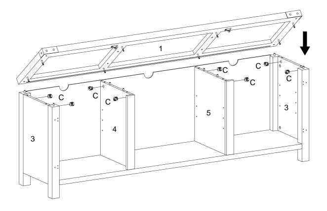
Insert part (1) into part (3,4,5), then insert and secure cam lock (C) to part (3,4,5).
