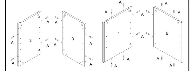
Insert wooden dowel (A) into parts (3,4,5)
