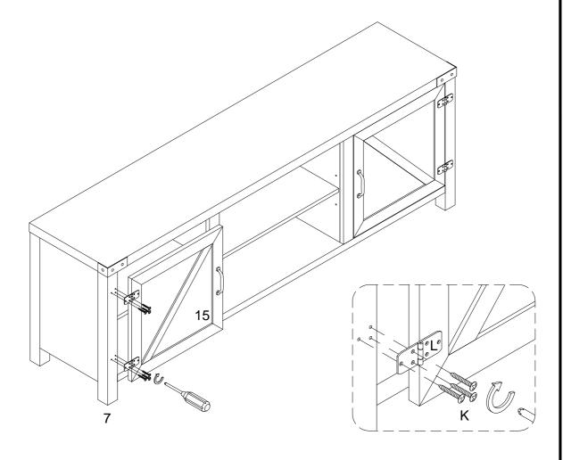
Using screw (K) with screwdriver secure the hinge and door and secure it door (15).
