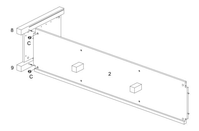
Attach part (8,9) to part (2), then insert and secure cam lock (C) to part (2) to lock it.
