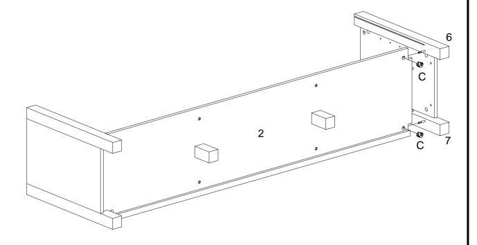
Attach part (6,7) to part (2), then insert and secure cam lock (C) to part (2) to lock it.
