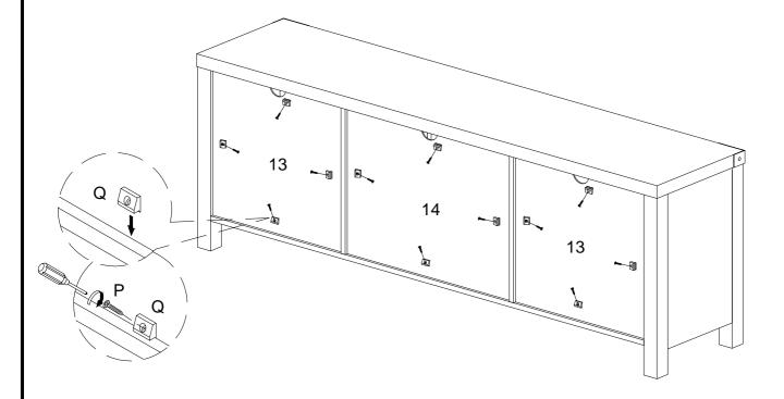
Secure plastic wedge (Q) to back panel (13,14) using screw (P) with screwdriver.
