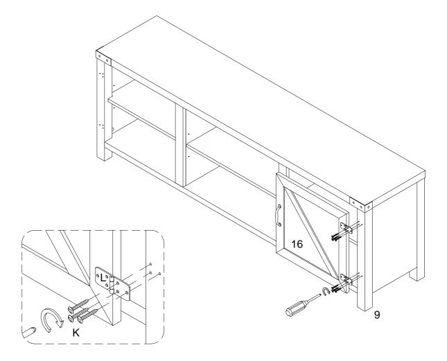
Using screw (K) with screwdriver secure the hinge and door and secure it door (16).
