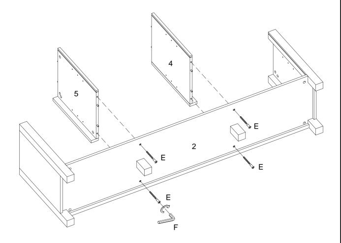
Attach part (2) to parts (4,5) using bolt (E) with hex key (F).
