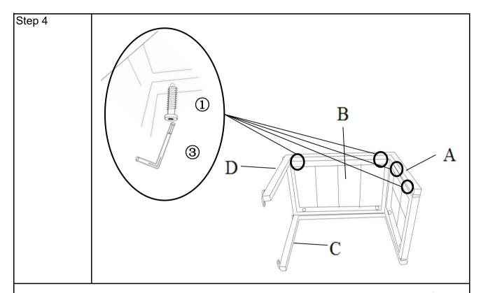
Attach the Left Side Support Bar(D) to Top Panel(A) and Side Panel(B) using Bolts( $\bigcirc$ ) with Allen Key( $\bigcirc$ ) as shown above.
