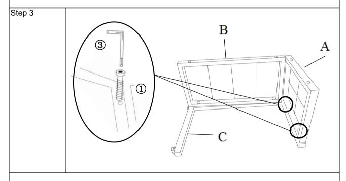
Attach the Top Panel(A) to Right Side Support Bar(C) and Side Panel(B) using Bolts( $\bigcirc$ ) with Allen Key( $\bigcirc$ ) as shown above.
