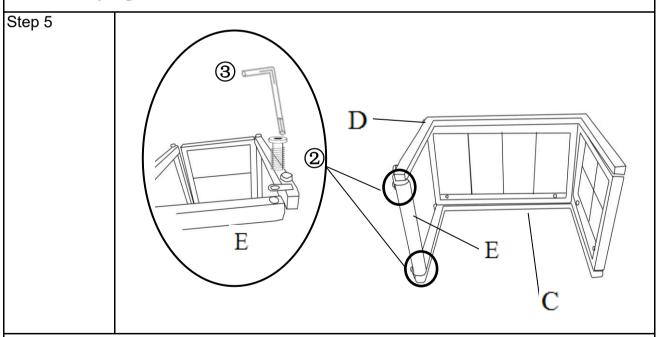
Attach the Horizontal Base Support Bar(E) to Right Side Support Bar(C) and Left Side Support Bar(D) using Bolts(2) with Allen Key(3) as shown above.
