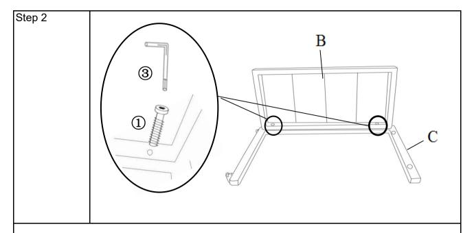
Attach the Side Panel(B) to Right Side Support Bar(C) using Bolts(1) with Allen Key(3) as shown above.
