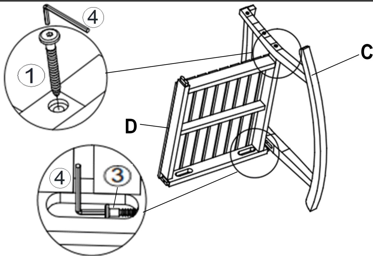
Align Seat Panel(D) with Left Leg Panel(C) as shown above.
