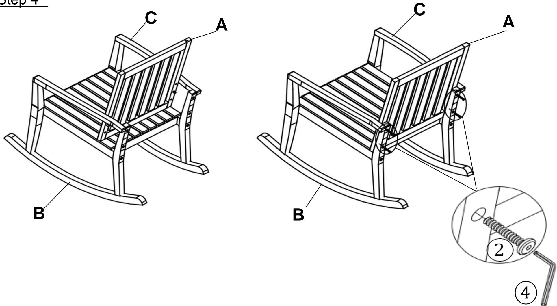
Attach Backrest Panel(A) to Right Leg Panel(B), Left Leg Panel(C), and Backrest Panel(A) using Bolts(②) with Allen Wrench(④).
