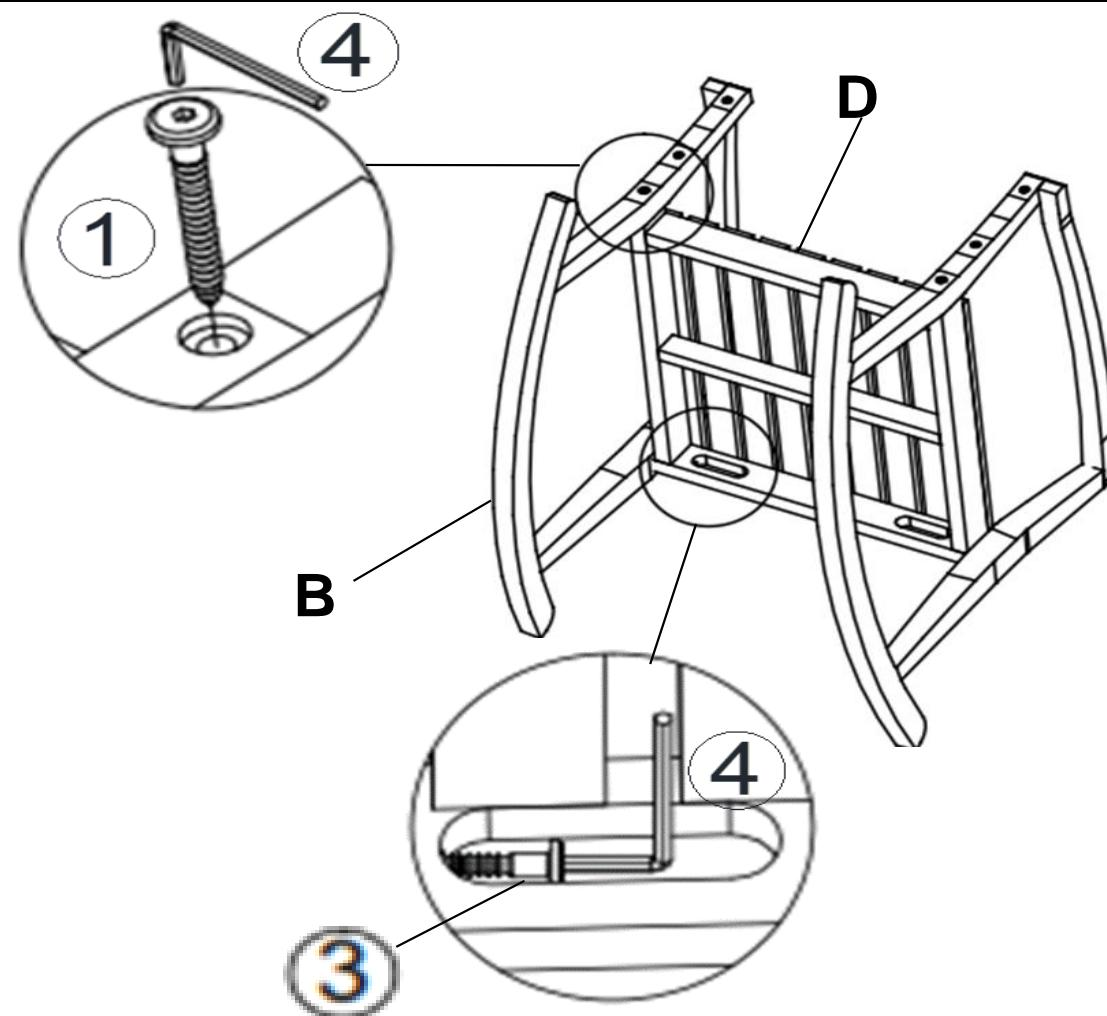
Align Seat Panel(D) with Right Leg Panel(B) as shown above.
