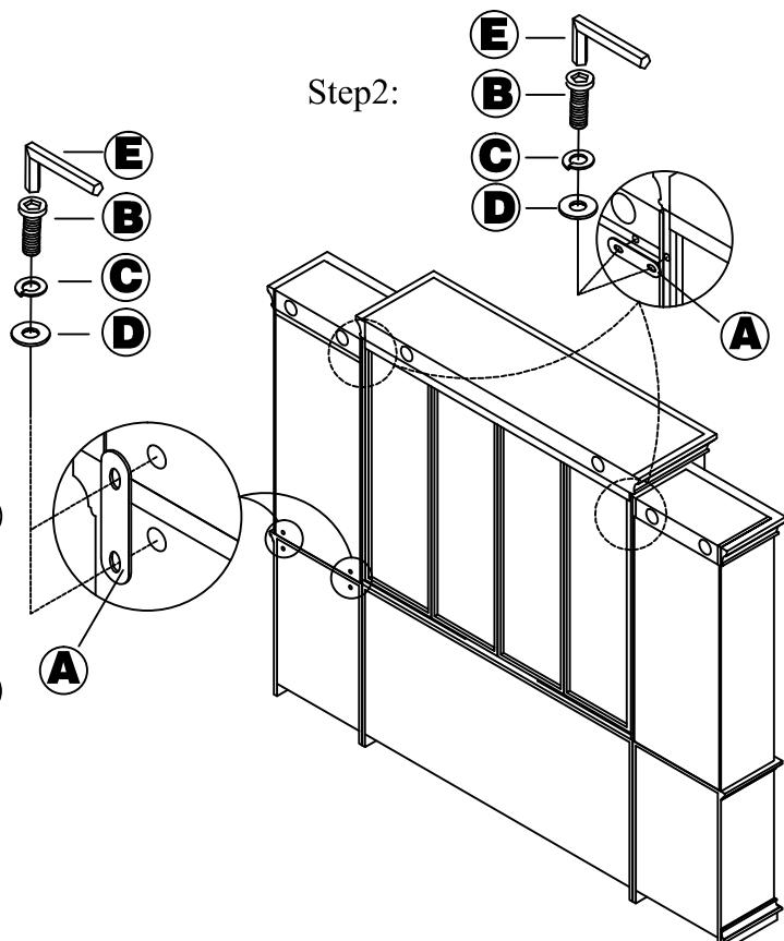
**NOTE: DO NOT TIGHTEN ALL THE BOLTS UNTIL THEY ARE INSTALLED IN CORRESPONDING HOLES!**
