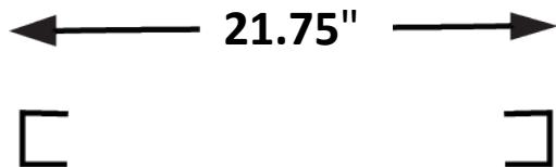
Using ground anchor installation layout drawing, dig holes 12" deep according to dimensions. Fill with cement and place ground anchors in wet cement. Be sure that ground anchors are straight and in accordance with dimension of ground anchor installation layout drawing. Allow cement to dry.
