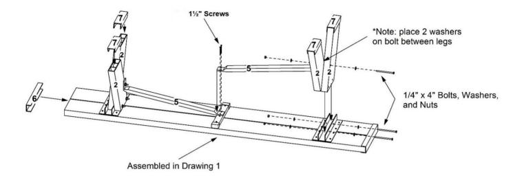
Insert one 15%" leg (part 2) into bracket. Place second 15%" leg (part 2) on inside of bracket and loosely fasten with 4" bolts, washers and nuts. Set 24%" diagonal brace on inside of legs with %" drilled hole against legs. Using one 4" bolt, washers and nut, fasten diagonal brace to legs.
