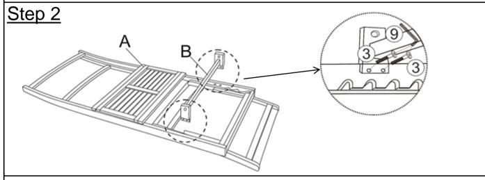
Place Seat Panel(A) facedown on a clean, non-marring surface. Position the Back Leg Panel (B) to Seat Panel (A) as pictured above by using Bolts (3) with Allen Key (9).
