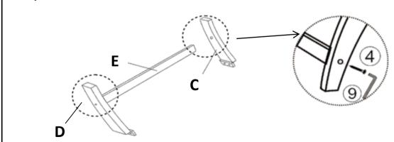
Attach Left Front Leg (C) to Leg Support Bar (E) by using Screws (4) with Allen Key (9).
