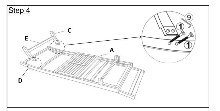
Attach the Pre-assembled in step 3 to Seat Panel (A) by using Bolts (1) with Allen Key (9).
