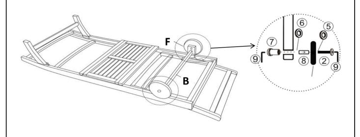
Attach one of Wheel (F) to Back Leg Panel (B) by using Bolt (2), Washer (5), Iron tube for Wheel (8), Washer (6) and Sleeve Nut (7) with Allen Key (9) in sequence as shown on the picture above.
