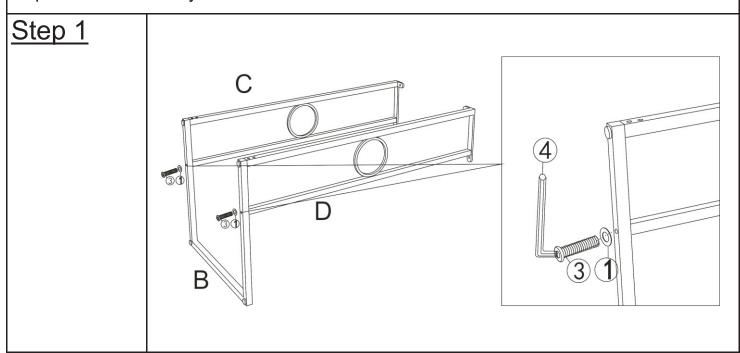
Place the Support Bar(B), Right Leg(C) and Left Leg(D) facedown onto a clean, non-marring surface.
