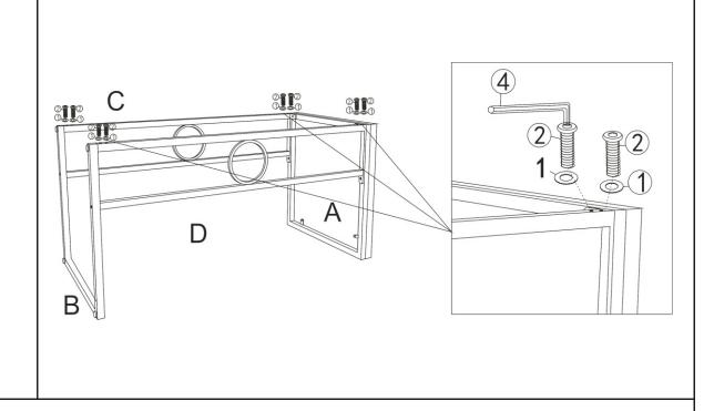
Attach Right Leg(C) and Left Leg(D) to Support Bar(B) using Washers(①) and Bolts(②) with Allen Key(④) as shown.
