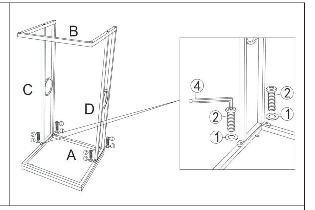
Attach Right Leg(C) and Left Leg(D) to Table Top(A) using Washers(1) and Bolts(2) with Allen Key(4) as shown.
