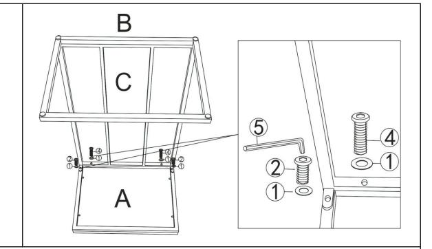
Align the mounting positions on the Table Top(A) and the Leg(C), Attach Leg(C) to Table Top(A) using Washer(1) and Bolt(4) with Allen Wrench(5) as shown.
