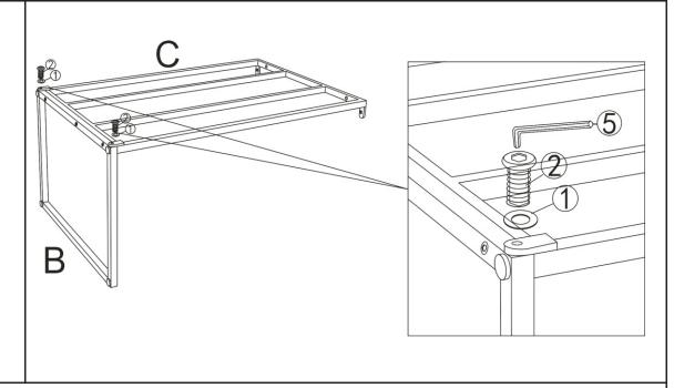
Attach Leg(C) to Support Bar(B) using Washer(1) and Bolt(2) with Allen Wrench(5) as shown.
