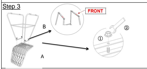
Align the mounting positions on Chair Leg(B) and Chair Seat(A), then attach using Nuts(1) with Spanner(2).
