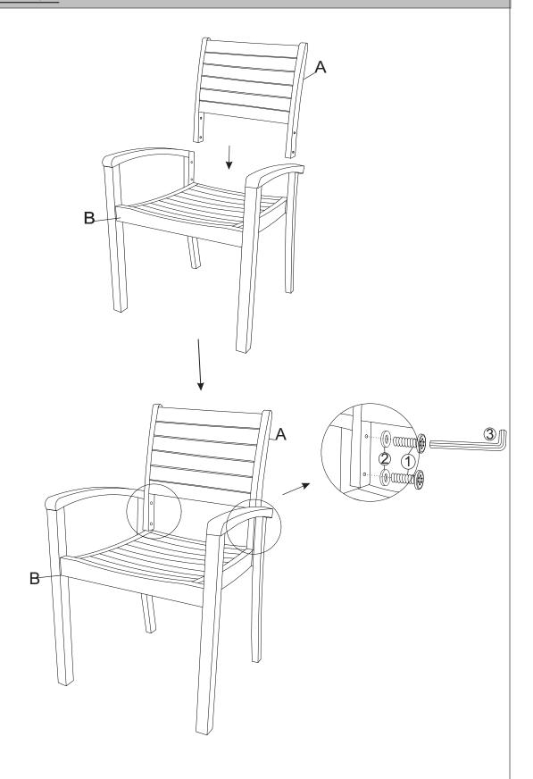
Position Backrest Panel (A) to the Seat Panel (B) as shown in picture above. Then affix Backrest Panel (A) with Seat Panel (B) by using Bolt (1), Flat Washers (2) and Allen Key (3).
