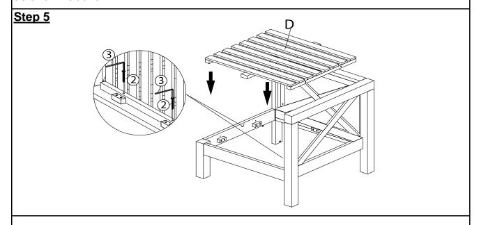
Attach the Seat Panel (D) into the Right Chair as shown in picture above. Affix Seat Panel (D) with Corner Chair by using Screws (2) and Allen Key (3). Note: Using Screws (2) from inside to outside of Seat Panel (D) **DO NOT FULLY TIGHTHEN SCREWS.**
