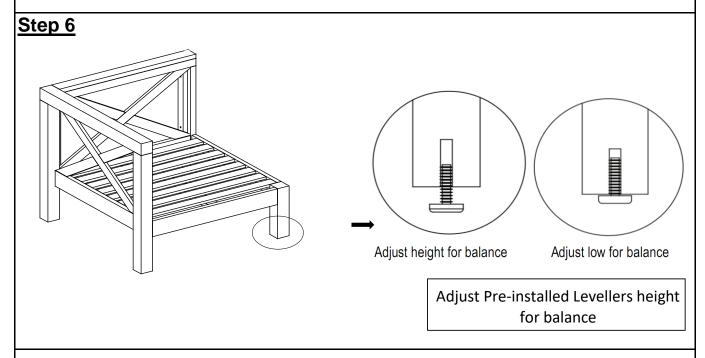
Inspect the Chair and make sure all parts are adequately connected. In a sequential manner, tighten all Screws and Bolts at all joints.
