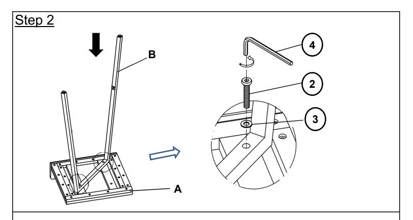
Position the Seat Panel(A) facedown on a clean, non-marring surface. Attach the First Leg Frame(B) to Seat Panel(A) using Bolts((2)), and Washers((3)) with Allen Key((4)).
