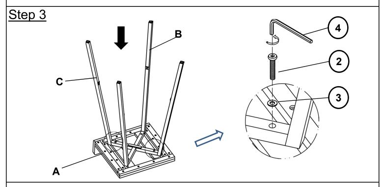
Attach the Second Leg Frame(C) to Seat Panel(A) using Bolts(②), and Washers(③) with Allen Key(④).
