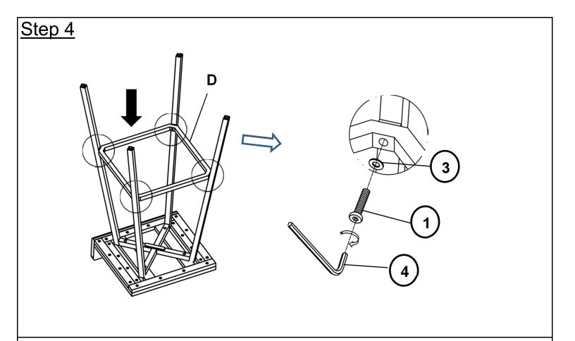
Align Leg Support Rail(D) between Legs, as shown above. Secure the Leg Support Rail(D) to the Legs using Bolts(1), and Washers(3) with Allen Key(4).
