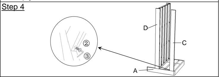
Connect the rear support rod (C) to the left panel (A) using an inner hexagon wrench (3) and bolts (2) as shown. Do not tighten the bolt completely.
