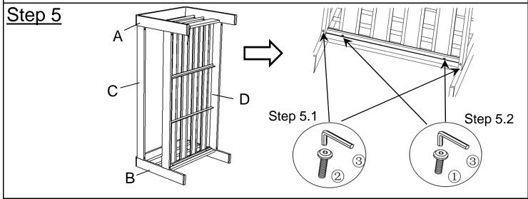
5.1)Attach Seat(D) and Right Side Panel(B) using Bolt(@) with Allen Key(@) as shown in the picture. 5.2)Attach Seat(D) and Right Side Panel(B) using Bolt(@) with Allen Key(@) as shown in the picture. Do not fully tighten the Bolt.
