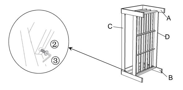
As shown, bolt (2) and connect the rear support rod (C) to the right panel (B) with an inner hexagon wrench (3). Loosen bolt not completely.
