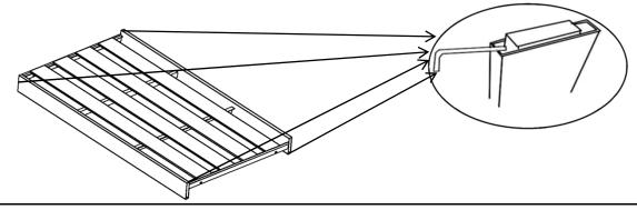
As shown above, use an inner hexagon wrench (3) to remove the plastic plug (to prevent aluminum deformation) from the four ends of the seat (D).
