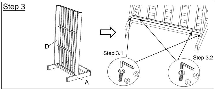
3.1)Attach Seat(D) and Left Side Panel(A) using Bolt(2) with Allen Key(3) as shown in the picture. 3.2)Attach Seat(D) and Left Side Panel(A) using Bolt(1) with Allen Key(3) as shown in the picture. Do not fully tighten the Bolt.
