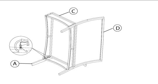
Place the Left Armrest/Leg(A) onto a clean, non-marring surface. Attach the Left Armrest/Leg(A) to Backrest(D) and Seat(C) using Bolts(2) and Washers(5) with Allen Key(1).
