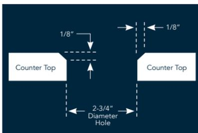
**Step 3.** Apply silicone to chamfer and mount sink to countertop using waste fitting and supplied Washer.
